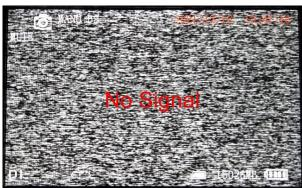
2. The LCD-12 monitor has been accidentally re-tuned to the wrong frequency
