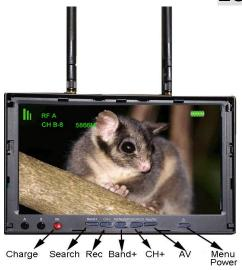
Turn **ON** your Nestbox Inspection Camera. With both antennas installed carefully fold open the sun shade, (*replacement shades are not available*). Hold down the **Menu/ Power** button release it when the LCD screen comes ON. Live video transmitted from the inspection camera should be visible with channel **CH - B-8** shown in top left of screen.
