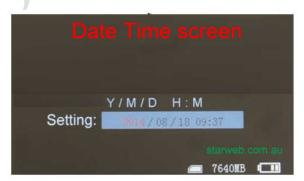
The display format is – Year – Month – Date – Hour – Minutes. The editable option will be highlighted in red. Use buttons 1 & 2 to increase or decrease the count then press button 5 to accept the change & move to the next option. Repeat the procedure for all the options.
